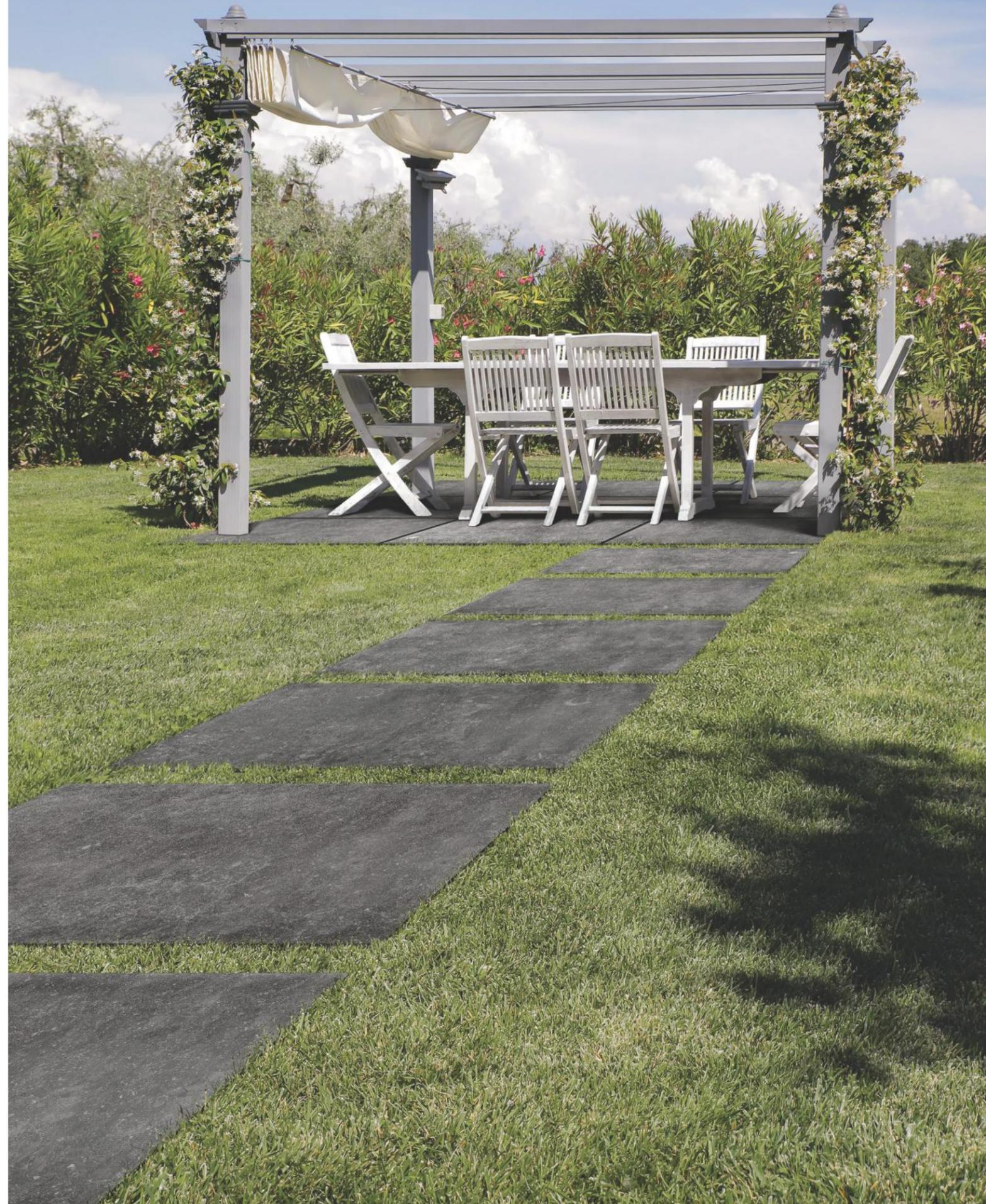
Landscape field tiles can be installed with a variety of methods, such as pedestal systems, sand setting, and typical mortar or thin set. For further questions/information about additional usages, please consult with your installer.
