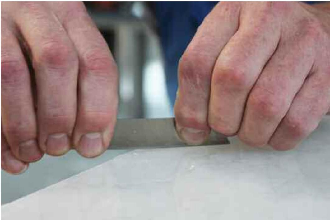
Clean the contact areas using Acetone before you apply the binder. This reduces the chance of small particles and dust affecting the glue and assists in the bonding.
