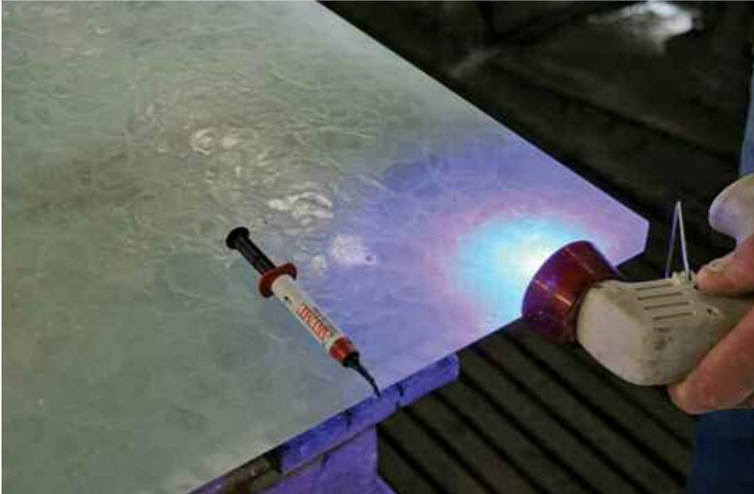
Then following this choice is **LOCTITE AA3491**. This is a transparent and thin flowing fill material which requires UV light hardening afterwards. This one offers the advantage of a short hardening time.
