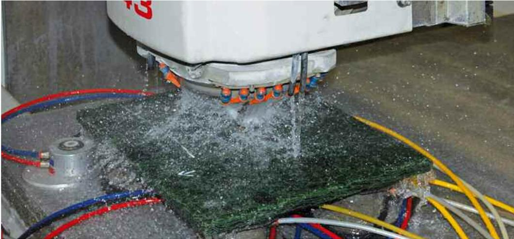
Generally we use two different methods of drilling holes. The first one is to drill through using waterjet, whereby you can vary the diameter.
