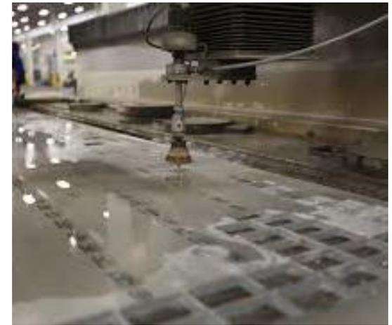
The lava stone tiles are cut into precise shapes, using a waterjet machine.
